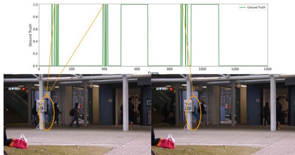
Fig. A.9. Continuity interruption (Video 1). The ground truth rapidly oscillates because of very brief occlusions caused by the pillars.
