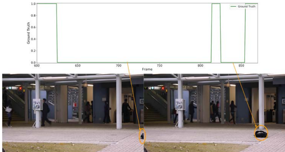
Fig. A.18. Static object mislabeling (Video 6). The backpack on the ground is considered normal, even though there is no instance similar to this in the training set.
