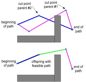
Figure 10: Example of the special crossover operator.
