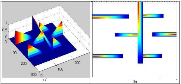
Figure 6-A Fuzzy map of an environment: 3D vision (a) and vision from the top (b).
