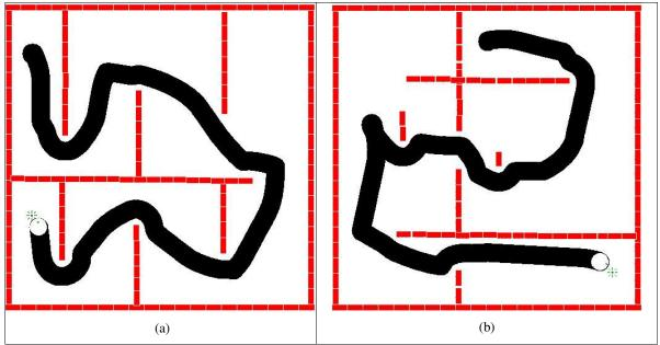
Figure 12 -Execution of the planned path in a complex environment (a), and with unknown obstacles (b).
