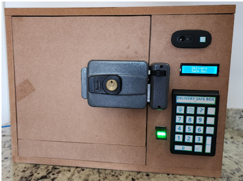
Figure 2: Mechanical Structure (To the left the main vault, to the right the control unit)
