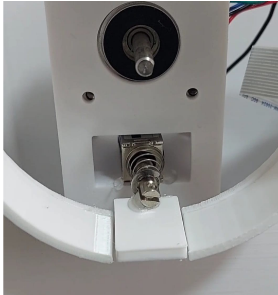
Figure 3: Internal view of the dispenser mechanism with motor and solenoid
