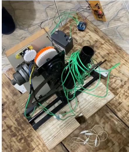
Figure 6: Gear responsible for radial movement coupled to mechanical arm
