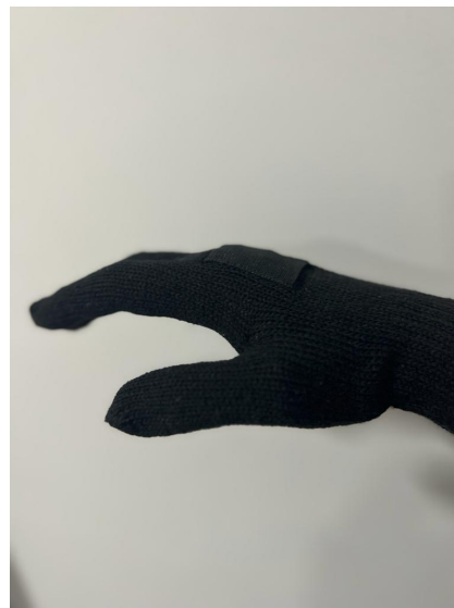
(b) Gyroscope Support sewn to the back of the glove (upper part)
