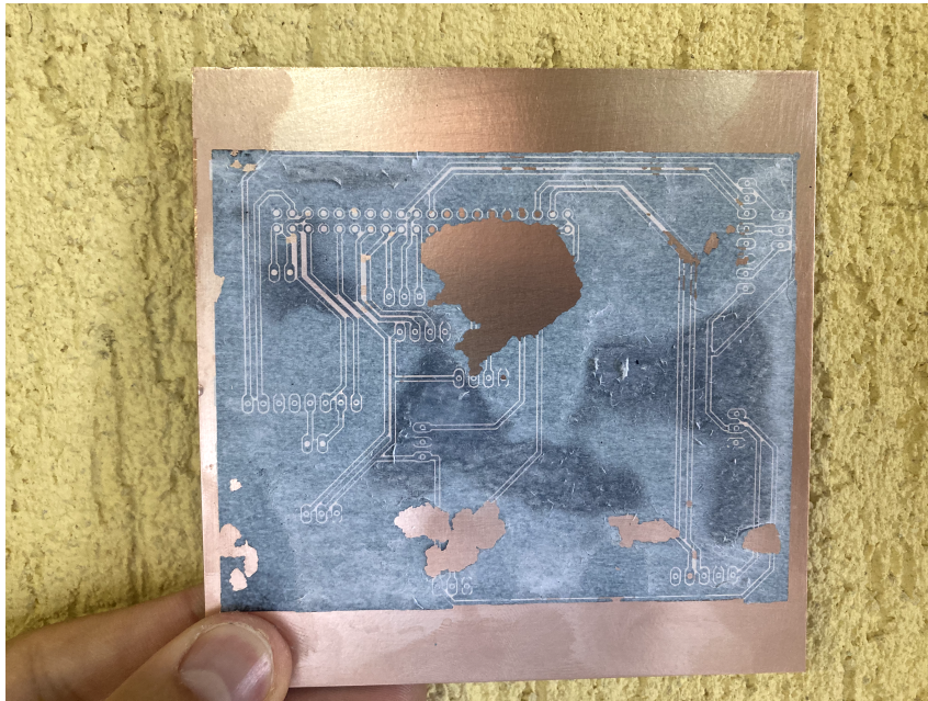
Figure 29: Failed attempt to transfer ink to copper board.
