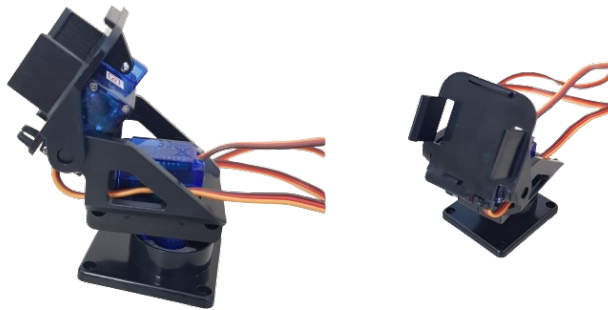
Figure 5: Structure for the camera and laser.
