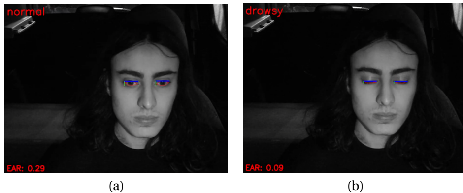
Figure 8: The bounding boxes of the eyes created in the algorithm. (a) Eyes are open, indicating normal state (b) Eyes are closed, indicating drowsy state
