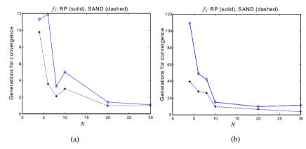
**Figure 21:** Average, over ten runs, of the number of generations for the GA convergence for randomly generated populations (RP) and populations diversified by the SAND algorithm with relation to the size of the initial set. (a) Function  $f_1$ . (a) Function  $f_2$ .
