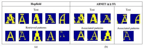
Figure 30: Results obtained for the Hopfield and ABNET algorithms. (a) The Hopfield network could not associate one of the independent patterns with its stored fundamental memories. (b) For  $\varepsilon \ge 55$ , the ABNET associated and grouped together two sets of the independent A patterns.
