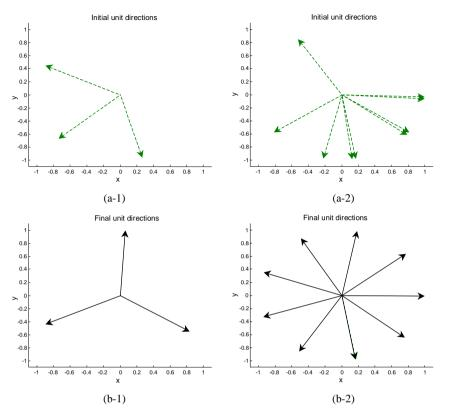
**Figure 19:** Generation of unit directions using the SA approach applied to Euclidean shape-spaces. The dashed arrows indicate the initial set of vectors (a), and the solid arrows represent the optimized vectors (b). (a-1, b-1) Three vectors (N = 3). (a-2, b-2) Nine vectors (N = 9).
