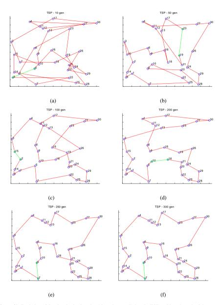
**Figure 41:** Evolution of the clonal selection algorithm when applied to the TSP problem. Length of the tours (in u.d.m. – unit of distance measure): (a) 107932, (b) 75627, (c) 60913, (d) 54540, (e) 49433 and (f) 48872.
