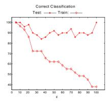
Figure 31: Generalization capability versus affinity threshold (ε) (Train and Test patterns presented in Figure 29).
