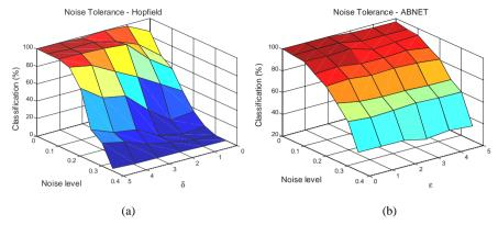
**Figure 28:** Noise tolerance of the Hopfield and ABNET.  $\delta$  is the allowed HD between the pattern recovered by the Hopfield network (a) and the stored pattern, and  $\epsilon$  is the affinity threshold of the ABNET (b).
