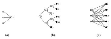
**Figure 25:** Constructing the network. Squares: input units; black circles: remaining cells; circles: cloned cells; dashed circle: pruned cell. (a) The initial network. (b) Network growing and pruning (input connections are omitted). (c) Resultant network architecture with its labeled cells.
