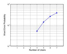
Figure 34: Major logic decision performance for a system with Q = 7 and L = 3. The word error probability represents the probability of correctly decoding the sent messages, and is equal to 0 for a number of users less than 4.
